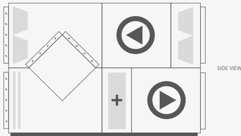
**10** supply & exhaust AHU with cross flow heat exchanger & heat pump module
