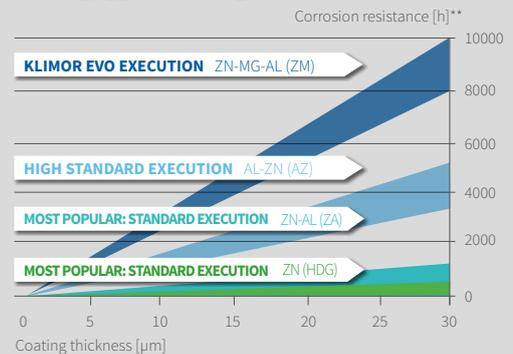
The source data: manufacturer, surface treatment: Zn (HDG), Zn-Al (ZA), Al-Zn (AZ), Zn-Mg-Al (ZM)
