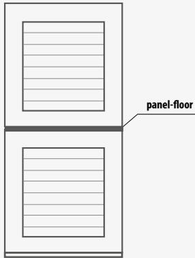
Standing one on another supply and exhaust unit sizes 0020=0021 are made as horizontal monoblock.
