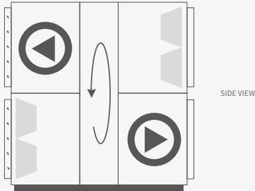
**2** supply & exhaust AHU with counter flow heat exchanger
