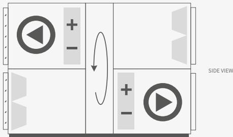
**4** supply & exhaust AHU with counter flow heat exchanger & gas module
