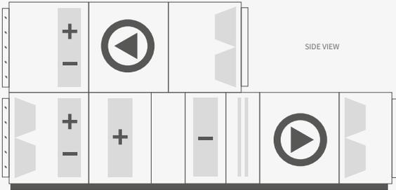
**8** supply & exhaust AHU with one-stage heat recovery (recirculation)
