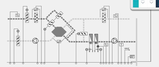
Monitoring of ambient, supply, exhaust and room temperatures / Monitoring of filter contamination / Monitoring of heat pump cooling system / Monitoring of fan unit operation / Air capacity control / Supply air temperature control / Energy recovery control / Frost protection for heat recovery exchanger and water heater / Free-cooling operation / Night recirculation of "fast heating"
