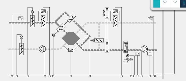
Monitoring of ambient, supply, exhaust and room temperatures / Monitoring of filter contamination / Monitoring of heat pump cooling system / Monitoring of fan unit operation / Air capacity control / Supply air temperature control / Energy recovery control / Frost protection for heat recovery exchanger and water heater / Free-cooling operation / Night recirculation of "fast heating"
