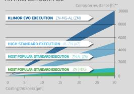
The source data: manufacturer, surface treatment: Zn (HDG), Zn-Al (ZA), Al-Zn (AZ), Zn-Mg-Al (ZM) \*\* The moment of red rust appearance on the given surface (salt spraytest)
