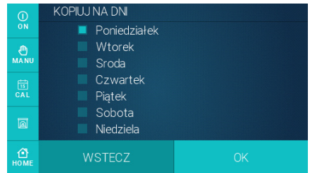
Fig. No. 38 Copying the calendar settings of the ADVANCE scheduler
