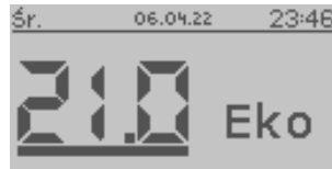
Fig. No. 27 STANDARD controller – main screen (temperature setting)
