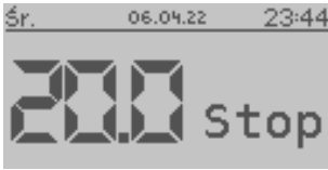
Fig. No. 23 STANDARD controller – active STOP mode
