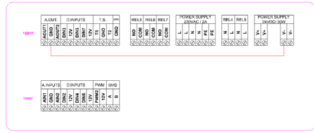
Fig. no. 11 Potential equalisation diagram of the terminal strip.
