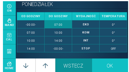
Fig. No. 37 Setting the calendar of the ADVANCE controller
