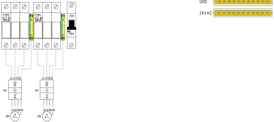
Fig. 58B Power supply diagram for 3-phases inverters 3x400VAC (eight fans below 11kW)
