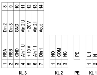
Fig. 27 Electrical connection diagram of a 1-phase EC fan
